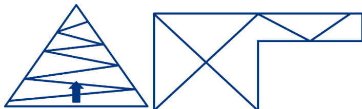
Figure 4b: combination of W, zigzag and cross pattern for collecting soil samples in oddly shaped areas
