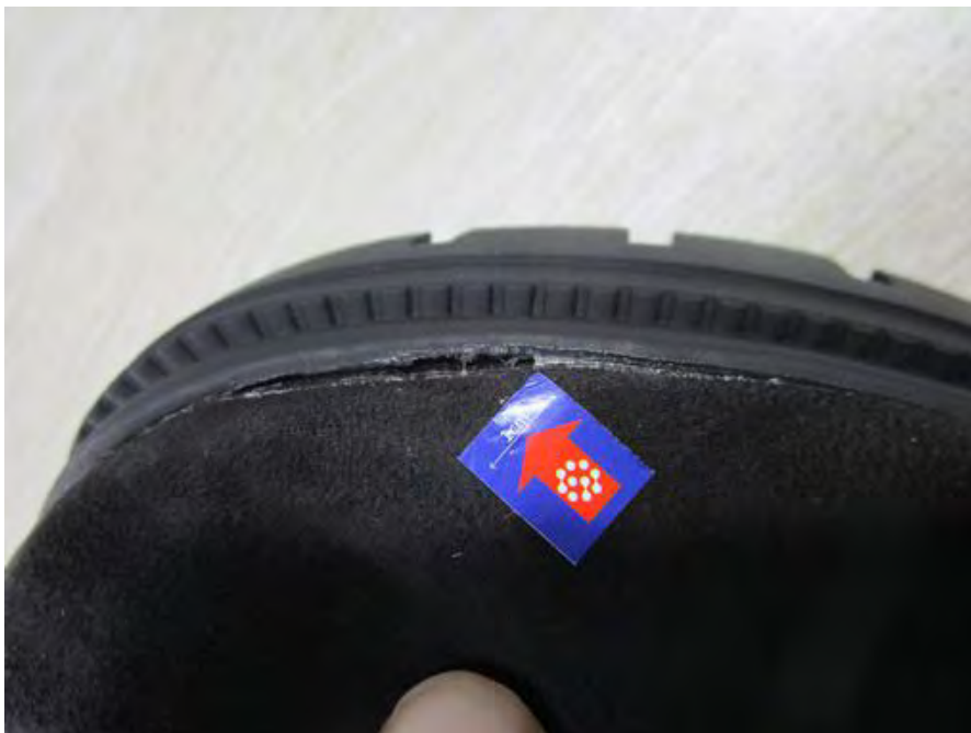
1 - D3 Weak cementing at second visual surface major 8
