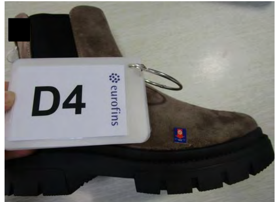
1 - D4 Glue mark at secondary visual surface major 5
