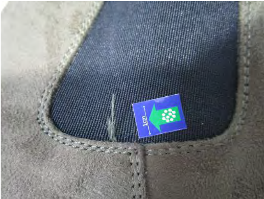
1 - D1 Uncut thread at primary visual surface minor 4
