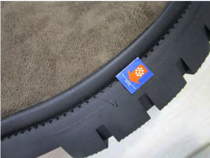
1 - D4 Glue mark at secondary visual surface major 4
