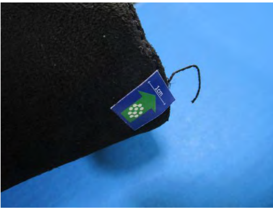
1 - D1 Uncut thread at primary visual surface minor 2
