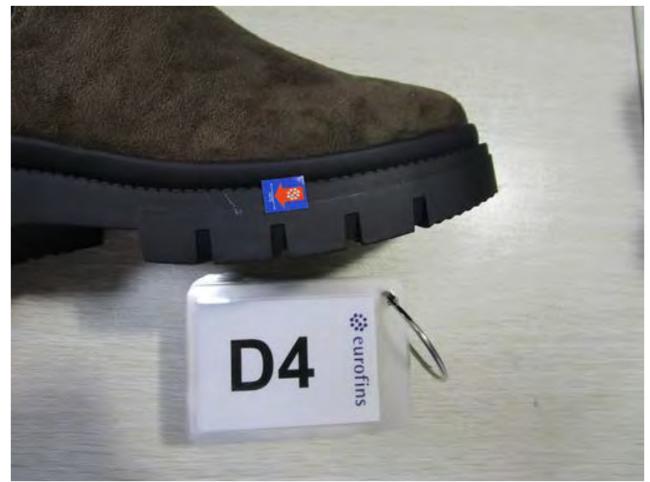
1 - D4 Glue mark at secondary visual surface major 3
