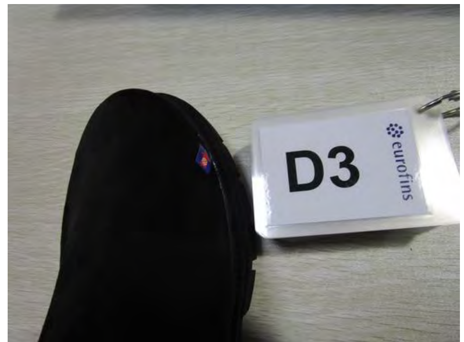
1 - D3 Weak cementing at second visual surface major 7
