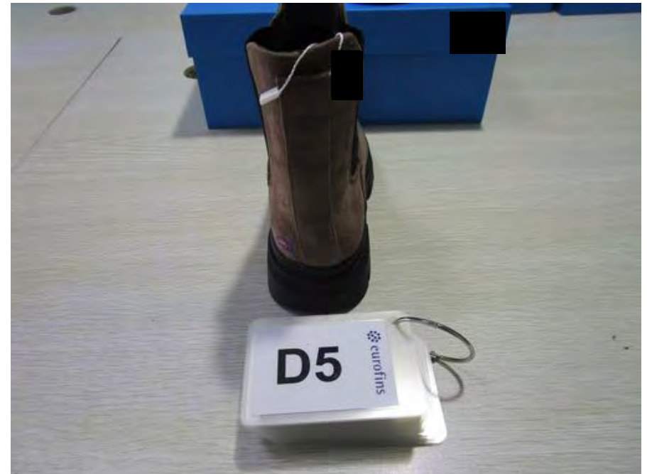
1 - D5 Counter off center at secondary visual surface major 3
