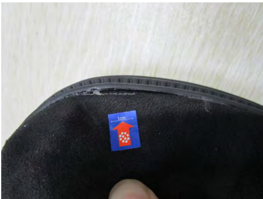
1 - D3 Weak cementing at second visual surface major 6
