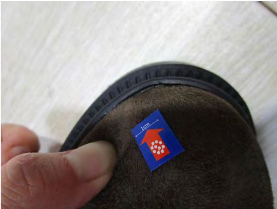
1 - D3 Weak cementing at second visual surface major 4
