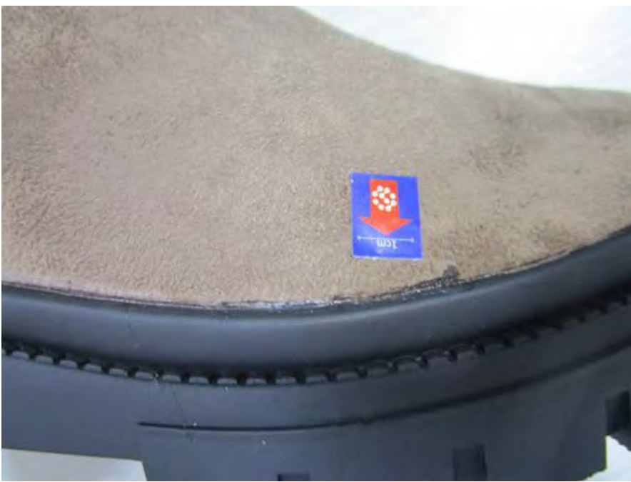
1 - D4 Glue mark at secondary visual surface major 6
