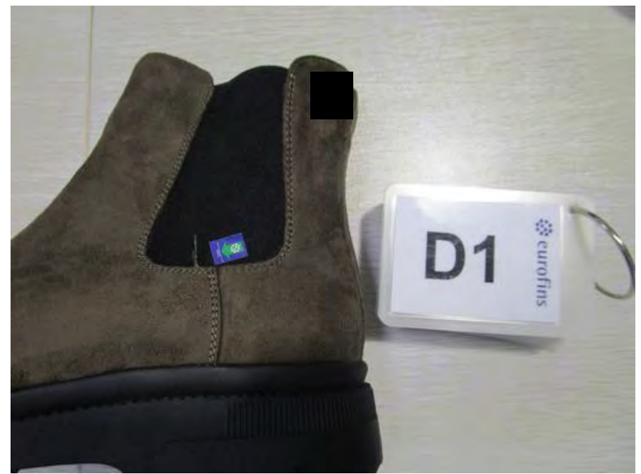
1 - D1 Uncut thread at primary visual surface minor 3
