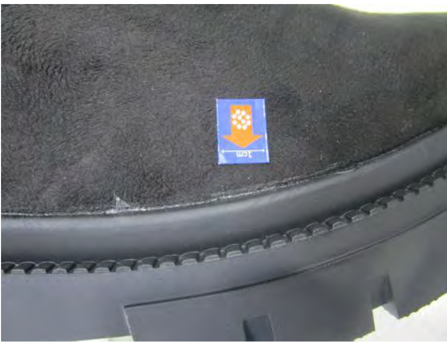
1 - D4 Glue mark at secondary visual surface major 2
