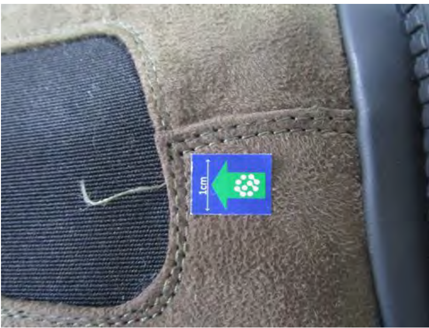
1 - D1 Uncut thread at primary visual surface minor 6
