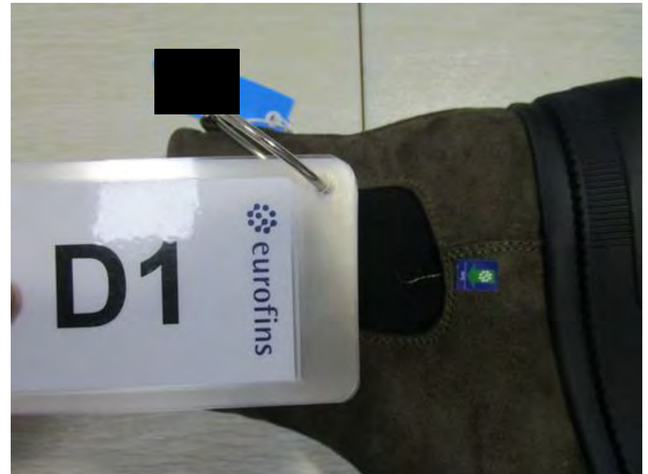
1 - D1 Uncut thread at primary visual surface minor 5
