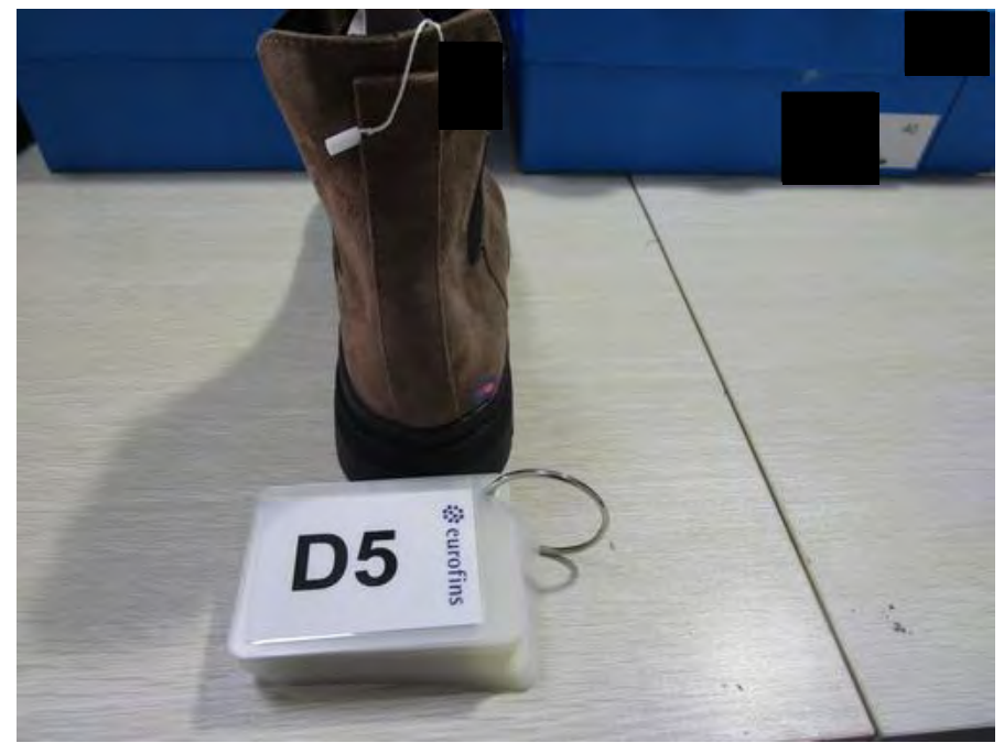
1 - D5 Counter off center at secondary visual surface major 1
