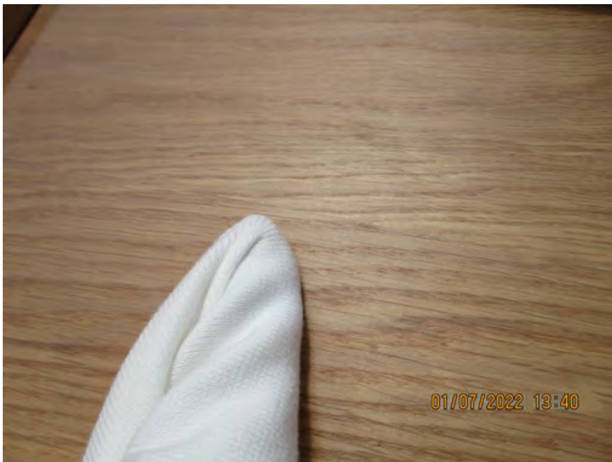
4.9 Product color resistance test (rubbing test with a dry tissue) 1
