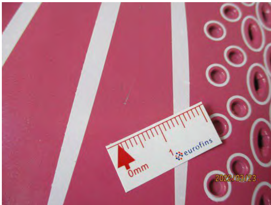
1 - D8 Scratch mark on the soleplate-minor 3
