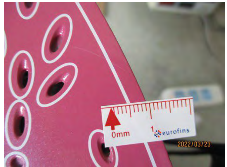
1 - D8 Scratch mark on the soleplate-minor 2
