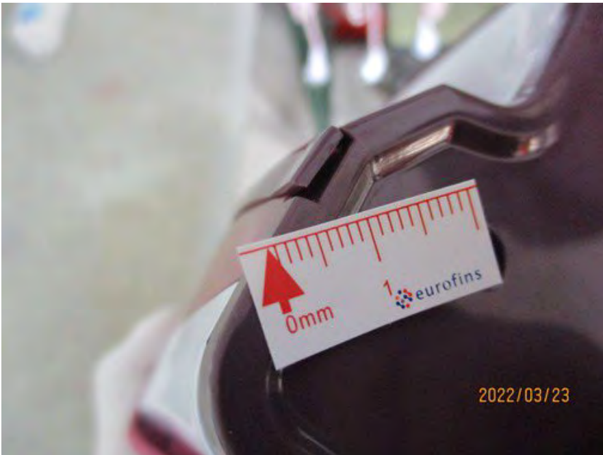
1 - D5 Poor assembly on the unit-minor 1
