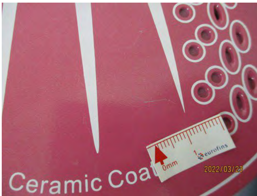
1 - D8 Scratch mark on the soleplate-minor 1
