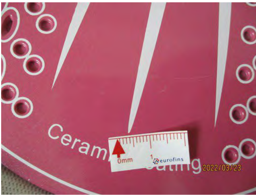
1 - D8 Scratch mark on the soleplate-minor 5
