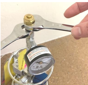
Figure 4. Removing brass cap
