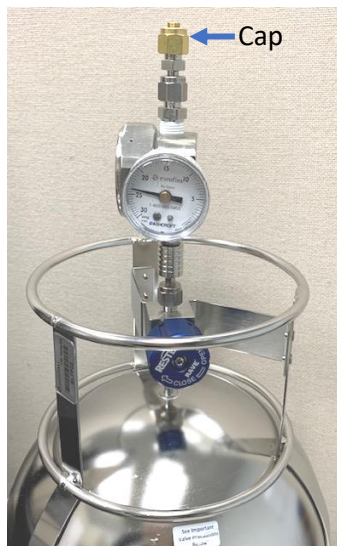
Figure 3. Pre-sample Vacuum check
