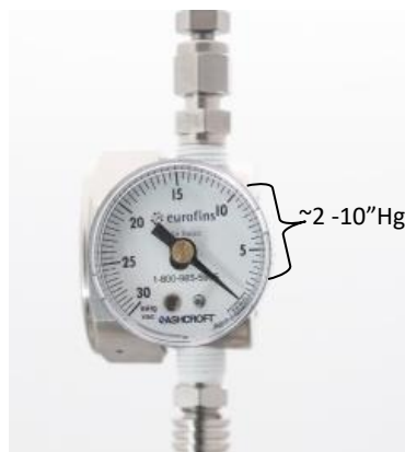
Figure 5. Record final field vacuum
